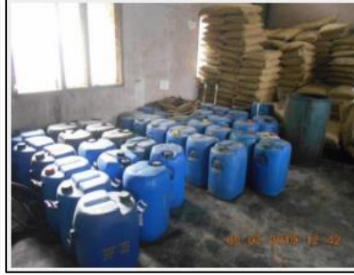
Non-compliance: No secondary containment for chemicals 化学品没 有二次容器
